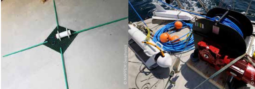
Fig. 52. Photographs of the STATEM (left) and PASSEM (right) systems prior to deployment at sea.
