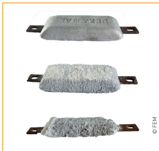
Fig. 1 : A galvanic anode at different stages of degradation.
