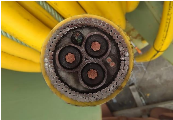
Fig. 4: Subsea cable internal composition (© France Energies Marines)
