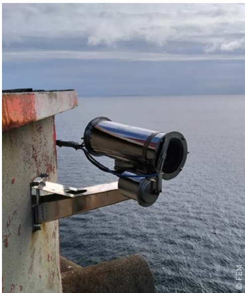
| Left-hand camera of the stereo-video system installed at the top of the lighthouse
