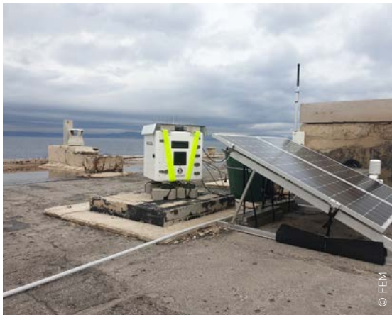
| Vaisala WindCube v2.1 profiling lidar deployed on Planier Island
