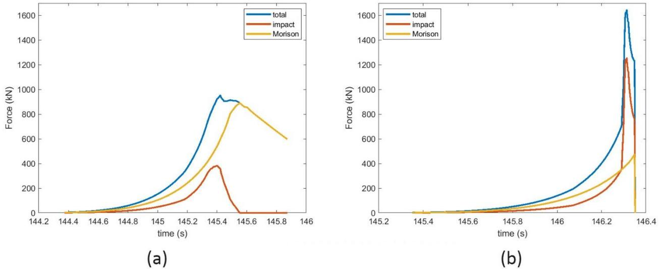
Figure 6. "Morison" loads, "Impact" load et total loads on the cylinder n°1 (a) and on the cylinder n°3 (b)
