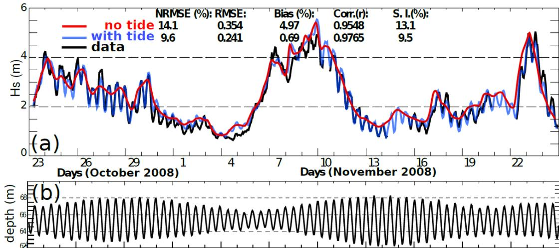
Figure 2. Sensitivity of wave forecasting by spectral model to the tidal current at buoy 62069 located at Pierres Noires, Brittany (from Ardhuin *et al.*, 2012)
