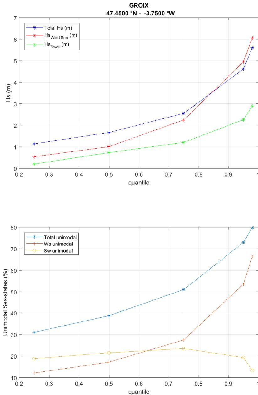
**Figure 3. Distribution of unimodal sea state conditions. Top figure: Significant wave height associated with quantiles for the complete sea states (Total), the wind sea component and the set of swell components (Swell). - Bottom figure: percentage of occurrence of unimodal sea states: All unimodal sea states (Total), unimodal wind sea only (Ws), unimodal swell only (Sw)**
