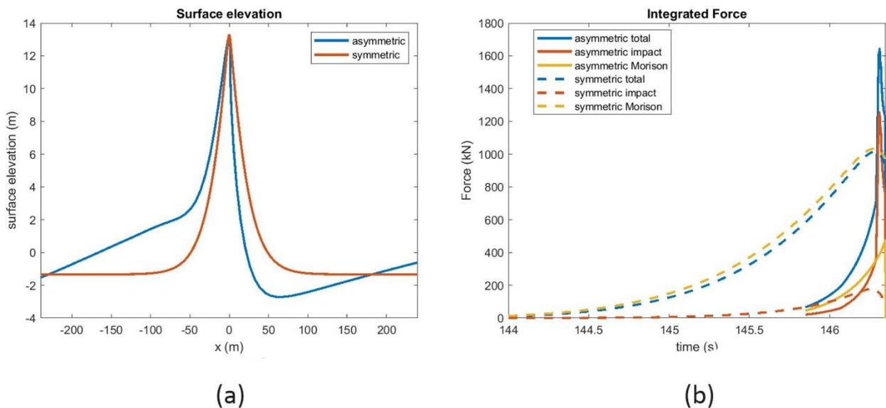
Figure 7. Symmetrical/asymmetrical wave comparison, regarding free surface elevation (a) and load of the offshore wind turbine (b)
