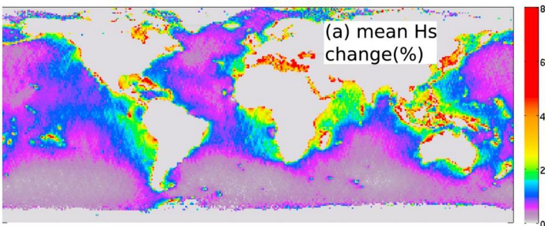
Figure 1. Effect of wave reflection at the coast on the significant height,  $H_s$  (from Ardhuin and Roland, 2012)
