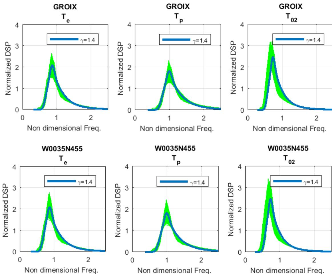
**Figure 4. Distribution of normalized spectra for extreme events (Groix site (top) - offshore site W0035N455 (bottom)) as a function of frequencies scaled by  $f_e$ ,  $f_p$  and  $f_{02}$  respectively**
