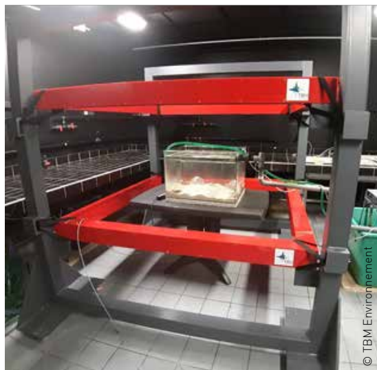
Fig. 39a: Helmholtz coils used for the experiments on great scallops.
