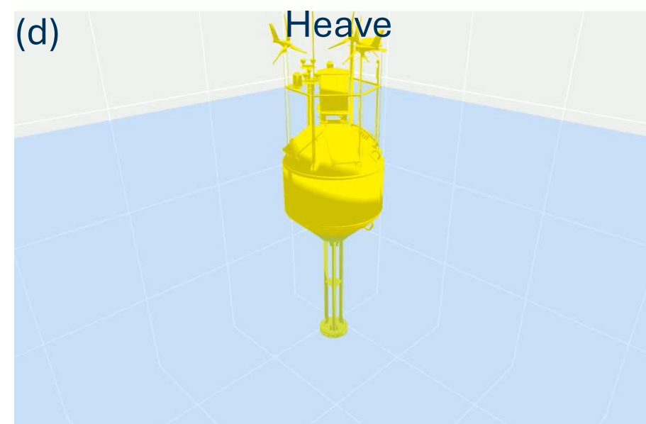
Animation showing a schematic representation of the six-degrees of freedom. Panel (a) roll, (b) pitch, (c) yaw, (d) heave, (e) surge, (f) sway.
