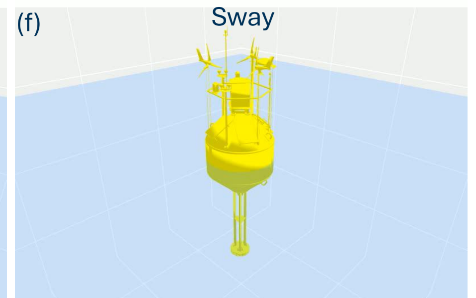
Animation showing a schematic representation of the six-degrees of freedom. Panel (a) roll, (b) pitch, (c) yaw, (d) heave, (e) surge, (f) sway.
