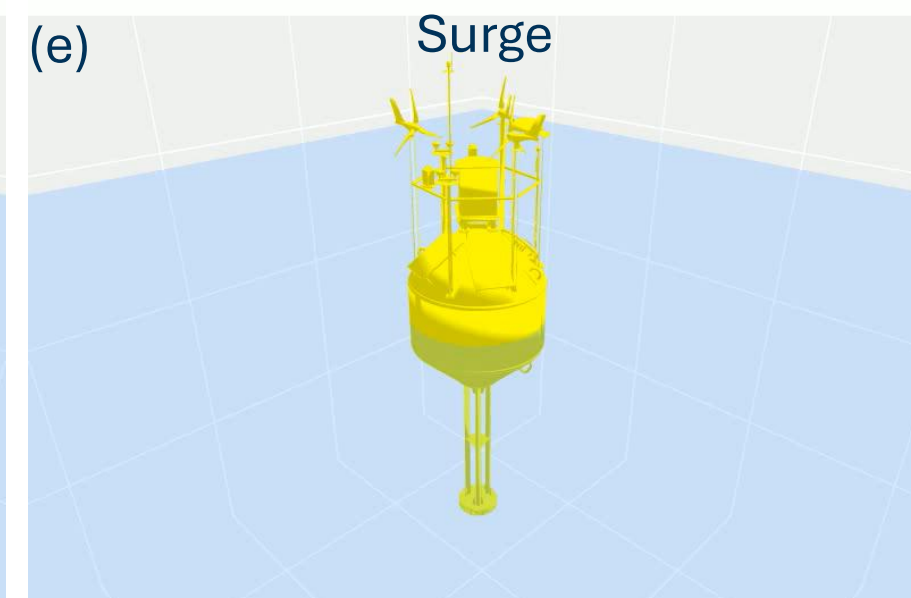
Animation showing a schematic representation of the six-degrees of freedom. Panel (a) roll, (b) pitch, (c) yaw, (d) heave, (e) surge, (f) sway.
