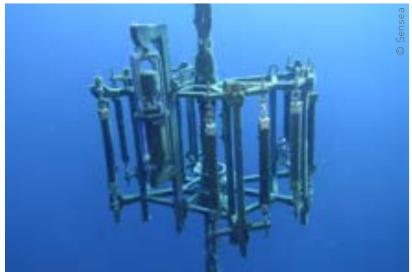
System comprising samples of high-density polyethylene (HDPE) and polyethylene terephthalate (PET) to monitor the biofouling of mooring lines and power cables and to quantify hydrodynamics
