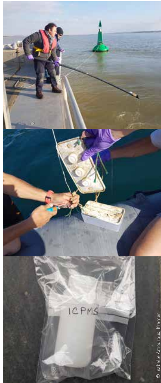
Figure 8. Illustration of water spot sample and DGT retrieval
