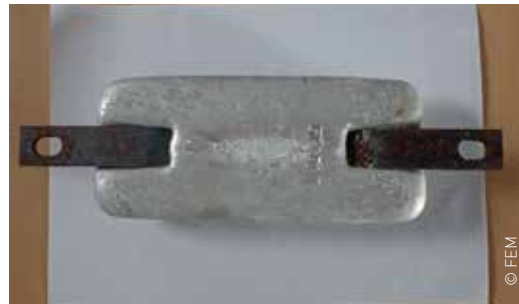
Figure 1. Example of galvanic anode cathodic protection
