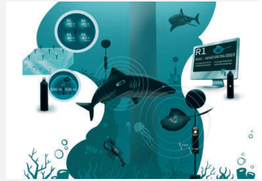
Fig. Conceptual illustration of passive acoustic telemetry methodology. Acoustic tags are placed on or within individual fish and crustaceans. Credit: ©FEM – Graphic creation by Lyna Couturier
