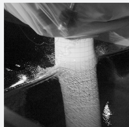
Slamming load on mockup, mounted on an hexapod to simulate floating offshore wind motions and tilt angles
