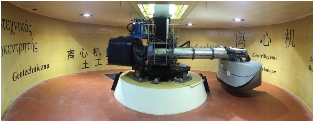
Centrifuge used for tests to investigate the behaviour of the anchorage under multidirectional and cyclic loads. Its radius is 5.50 m (© Université Gustave Eiffel)
