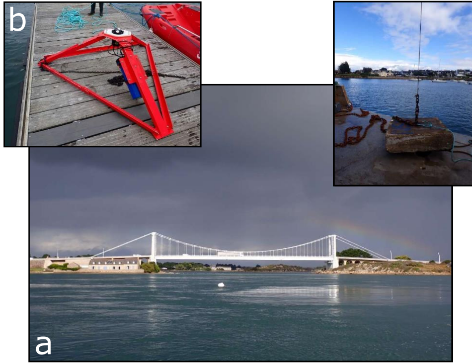
Figure 11. (a) Photograph of the Étel estuary test site with the Lorois Bridge in the background. The White surface buoy signals the location of the bottom-mounted Nortek Signature. (b) The Nortek Signature mounted on an aluminium tripod prior to its deployment in the Étel estuary. (c) 2.5 ton concrete mooring used to secure the tripod. The concrete mooring and the tripod were connected by a 10 m long, 8 cm width chain.
