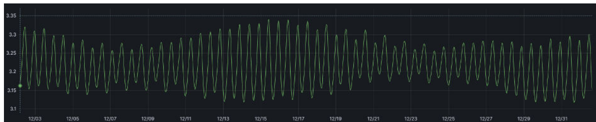
Figure 4: Pressure reading, in Bar, from the external pressure sensor on M100-D over one month
