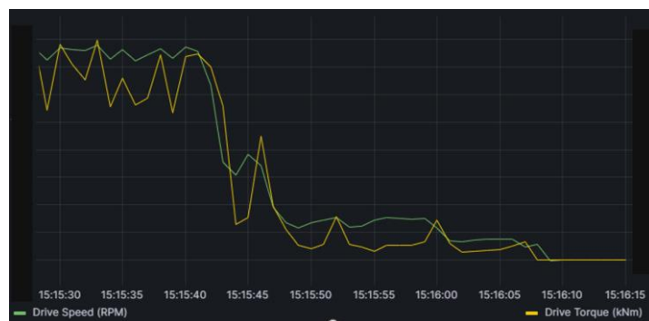
Figure 8: Speed and torque time series during the same grid loss event
