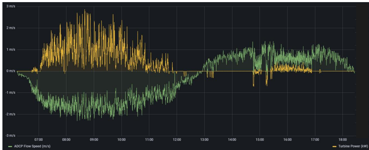
Figure 18: 30 Second Average Flow Speed and Turbine Output Power Time Series for a Typical Ebb and Flood Tide Cycle (Ebb Tide Shown with Negative Speed)
