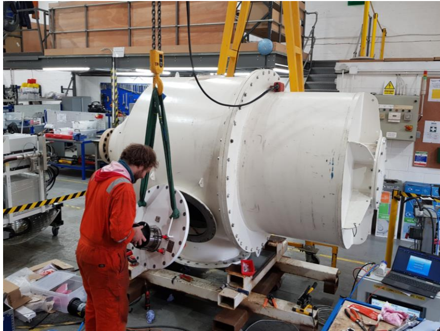
Figure 4: Installing the Turbine Waterproof Connector System
