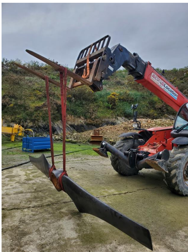
Figure 6: Displacement of the blade after being removed from the turbine
