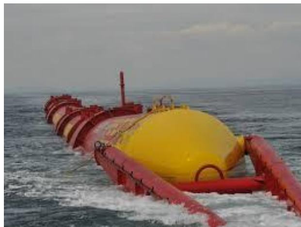
Figure 3.4.4-5:: Photo of the nose of the Pelamis P2 device and the yoke system used for towing and connecting to the mooring system [10]
