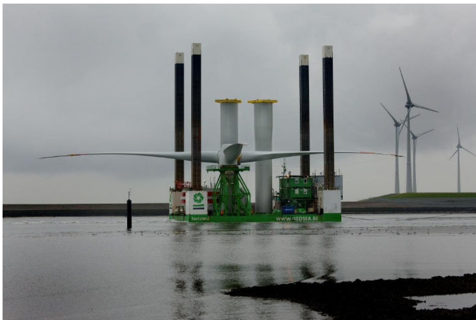
Figure 3.4.2-5: Transportation of Offshore Wind Turbine using jack-up barge Goliath [20]
