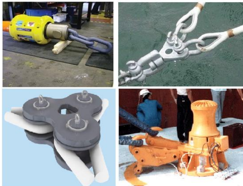
Figure 3.4.4-4: Example of connectors for mooring systems used in the Oil&Gas sector: rope to chain connector LankoFirst (top right), Bridle plate connection system
