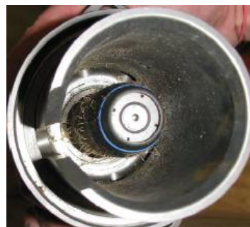
(b) marine growth on the inside of connector
