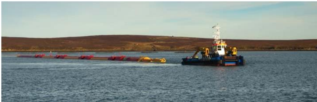
Figure 3.4.2-2: The Pelamis towed to site [10]
