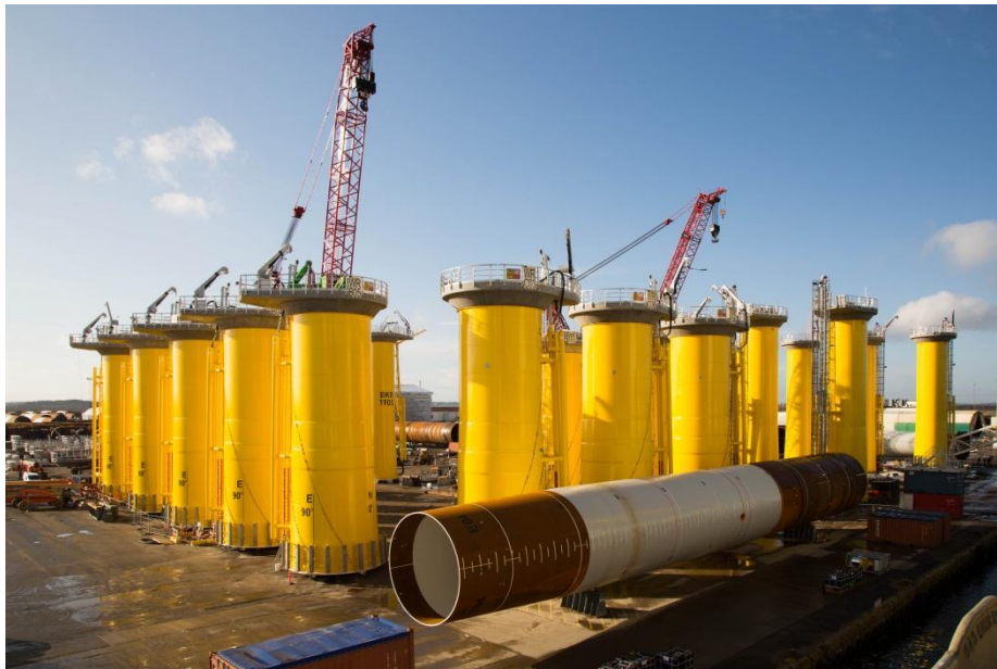
Figure 3.4.1-1: Example of sufficient inland area required for offshore wind transition pieces at Westernmost Rough [20]
