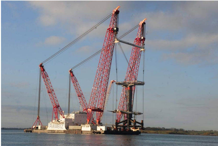
Figure 3.4.2-4: Transportation of MCT SeaGen S Mk1 and foundations to Strangford Lough, Northern Ireland [122]
