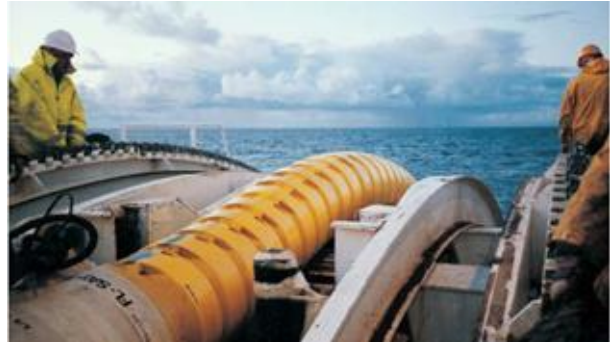
(b) overboarding bend stiffener using cable chute [49]
