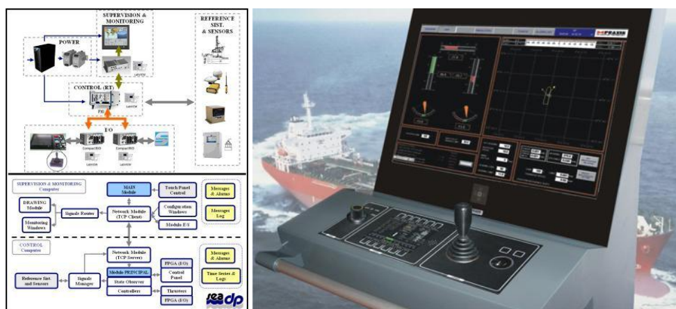
Figure 3.4.4-2: Working principle of a DP system and photo of the Praxis' DP system [132]
