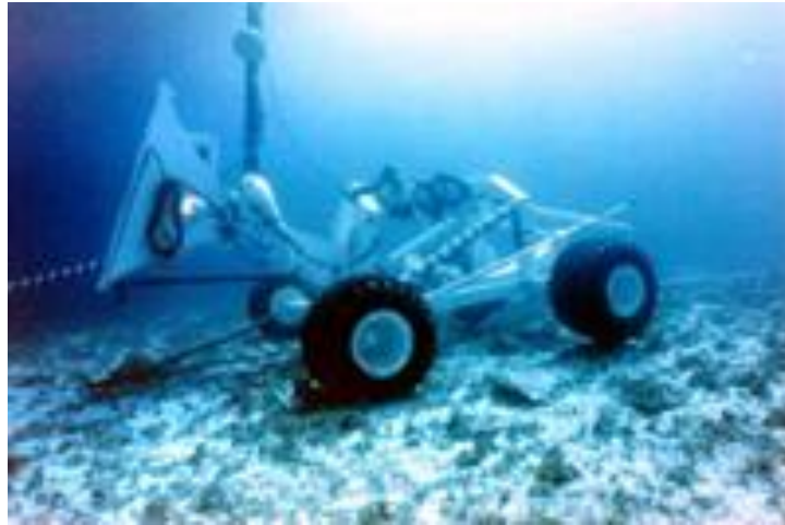
Figure 3.1.1-4: The HYDRO PLOW submarine trencher of Prysmian in operation [15]
