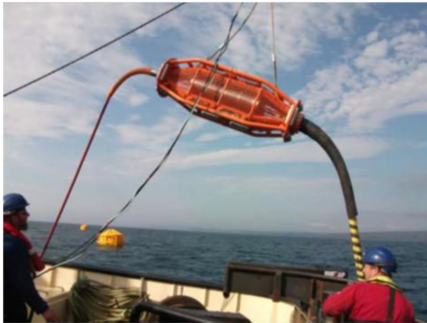
Figure 3.1.2-9: Returning Wello WEC connector to the seabed [43].
