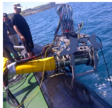
(b) umbilical cable and ROV being overboarded
