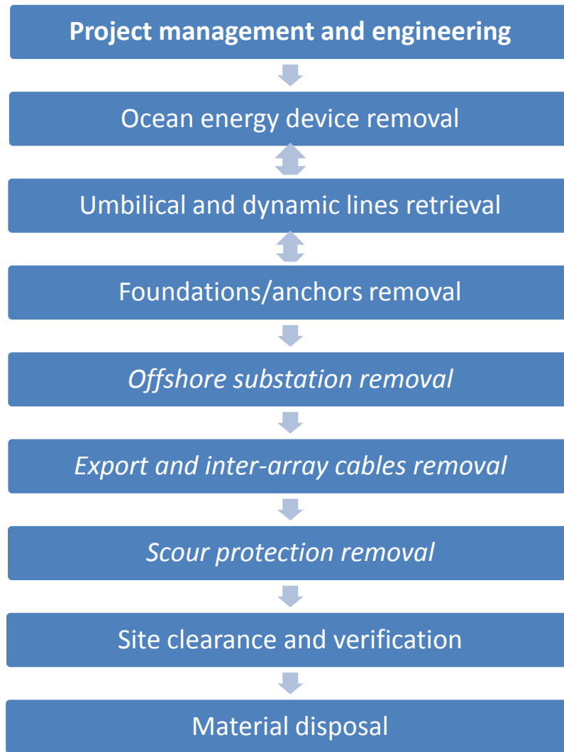
Figure 5-2 Summary flow chart of the key logistic steps occurring during the decommissioning phase of an MRE project
