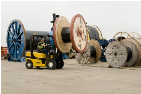
Figure 2.2.4-6: Example of subsea cabling storage structures: cable drums (on the left) and a turntable (on the right) [15]
