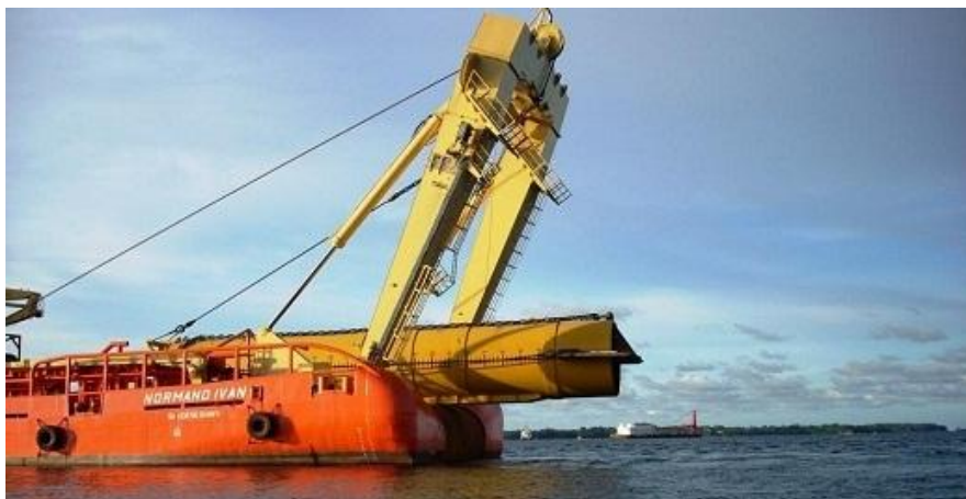
Figure 3.2.4-6: Direct embedment anchor attached to driver ready for deployment [86]
