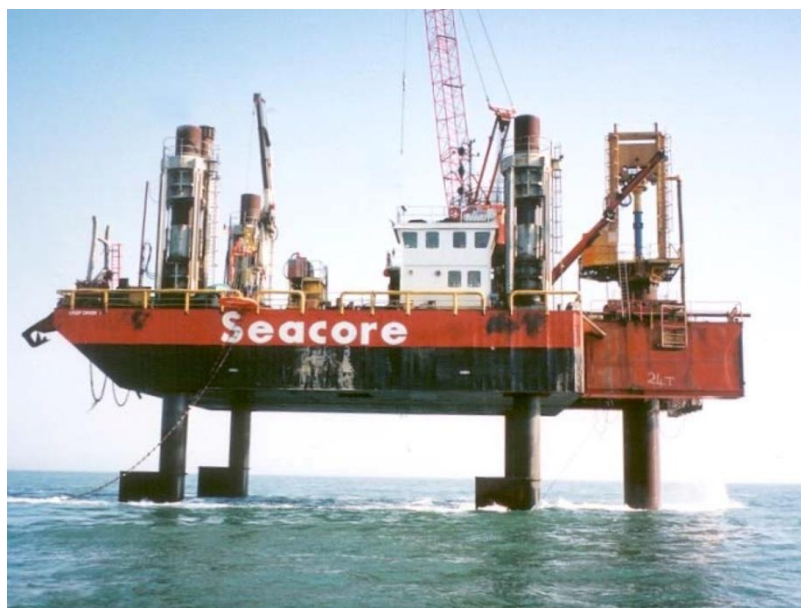
Figure 3.4.3-1- Deep Diver Seacore jack-up barge [127]
