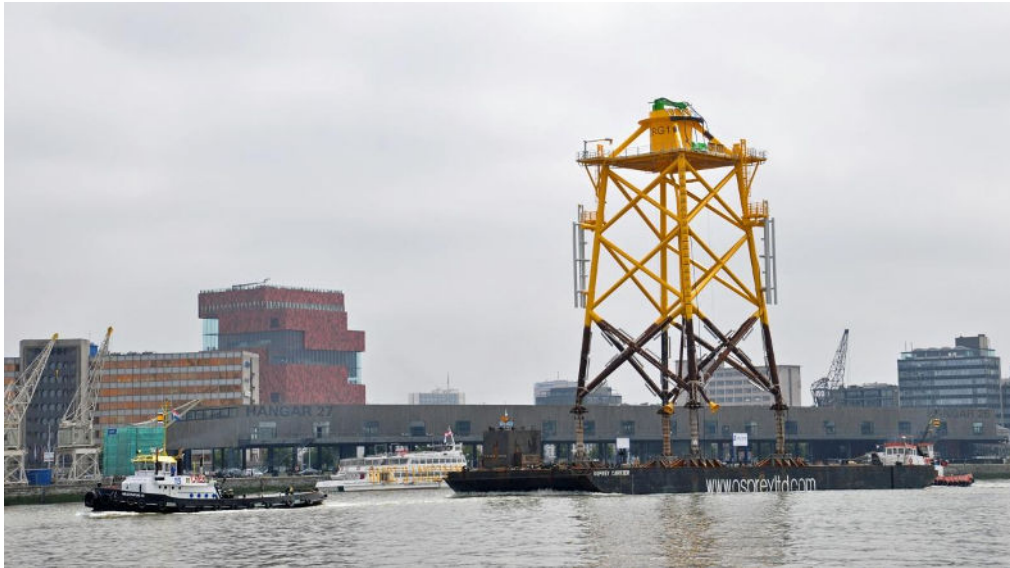
Figure 3.4.2-6: Transportation of Offshore Wind foundation jackets using barge [20]
