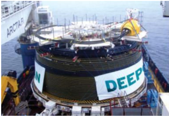
(a) unit on modified cable carousel [57]
