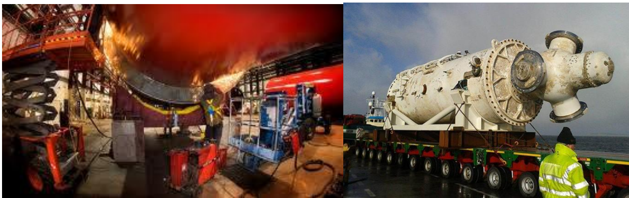
Figure 2.2.2-2: A technician attending one tubular section of the Pelamis machine (left) [10], steel hull structure of the Hammerfest tidal turbine being transported at port (right) [11]
