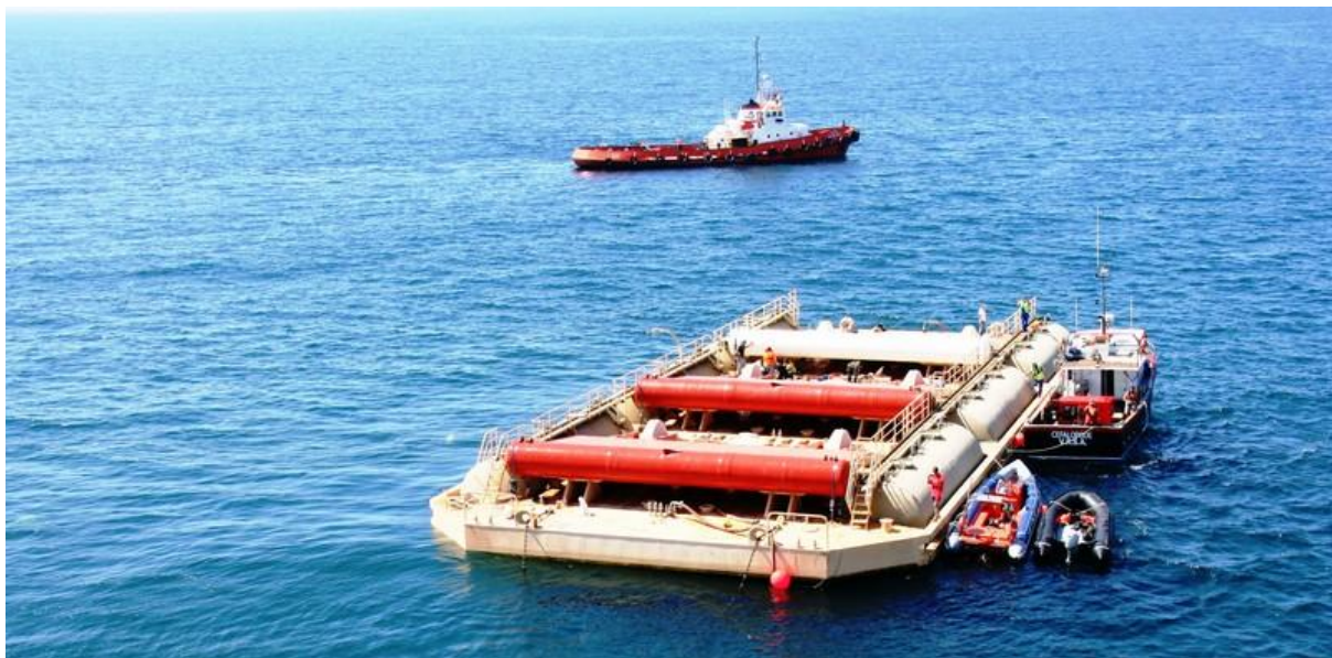
Figure 3.3.3-6: The WaveRoller wave energy converter, attached to the foundation structure which is sunk by flooding a number of ballast tanks on the sub-structure [117]
