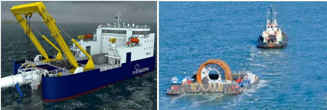
Figure 3.3.1-6: (left) HF4 vessel designed by Mojo Maritime [104][105] and (right) OpenHydro Installer barge [106]
