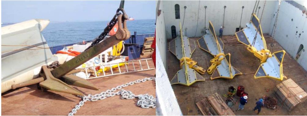
Figure 16: Anchor examples ( left ) 1.1 Tonne Danforth fluke anchor prior to deployment with the South West Mooring Test Facility (SWMTF, [43]), ( right ) vertically loaded Delmar OMNI-Max anchor
