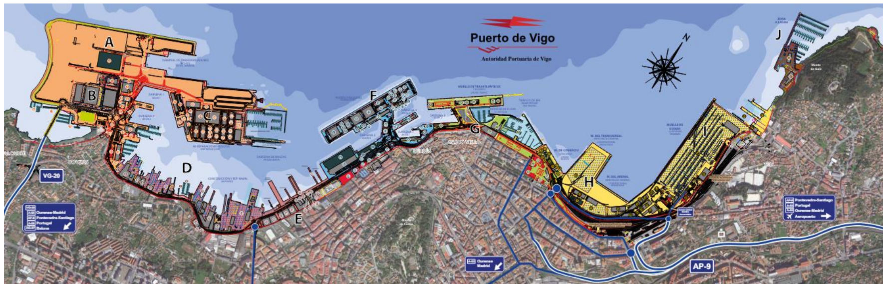
Figure 2. Map of the Port of Vigo. A: Ro-Ro terminal, B: free economic zone area; C: ship repair dock; D: shipyards; E: cold storage; F: fishing port; G: cruise facilities; H: commercial quays; I: container terminal; and J: Marina.
