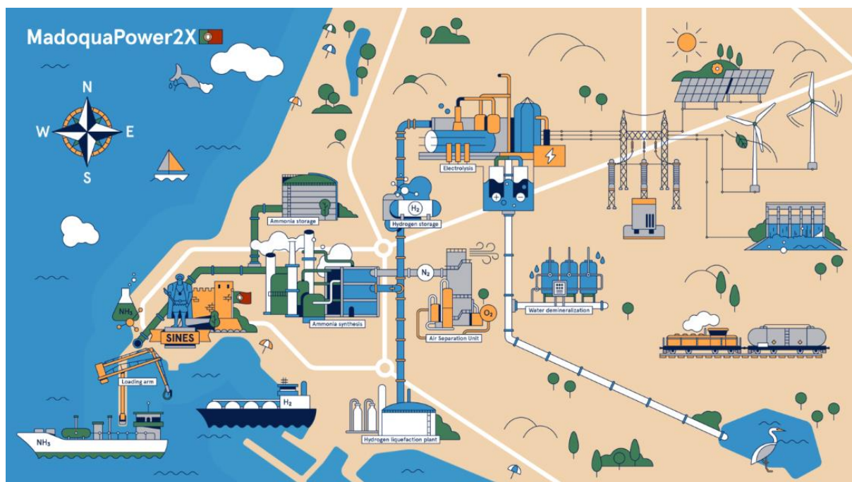
Figure 4 - The infrastructure required, and the process used to produce green Hydrogen and Ammonia.
