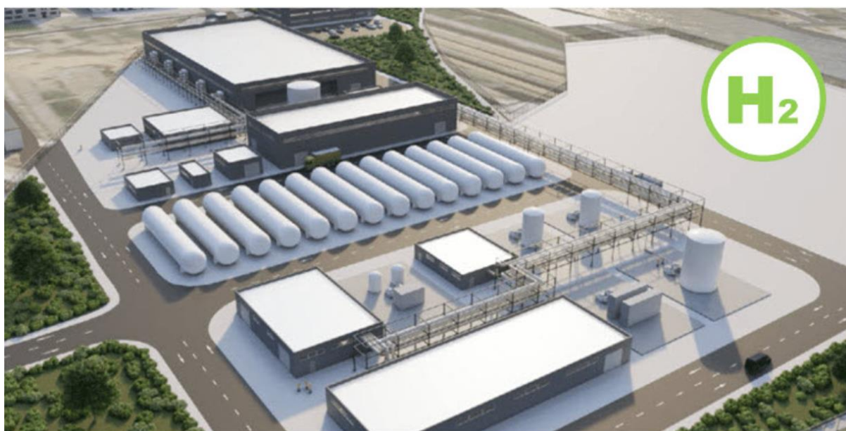
Figure 11 - 3D design of Hydrogen production facility.
